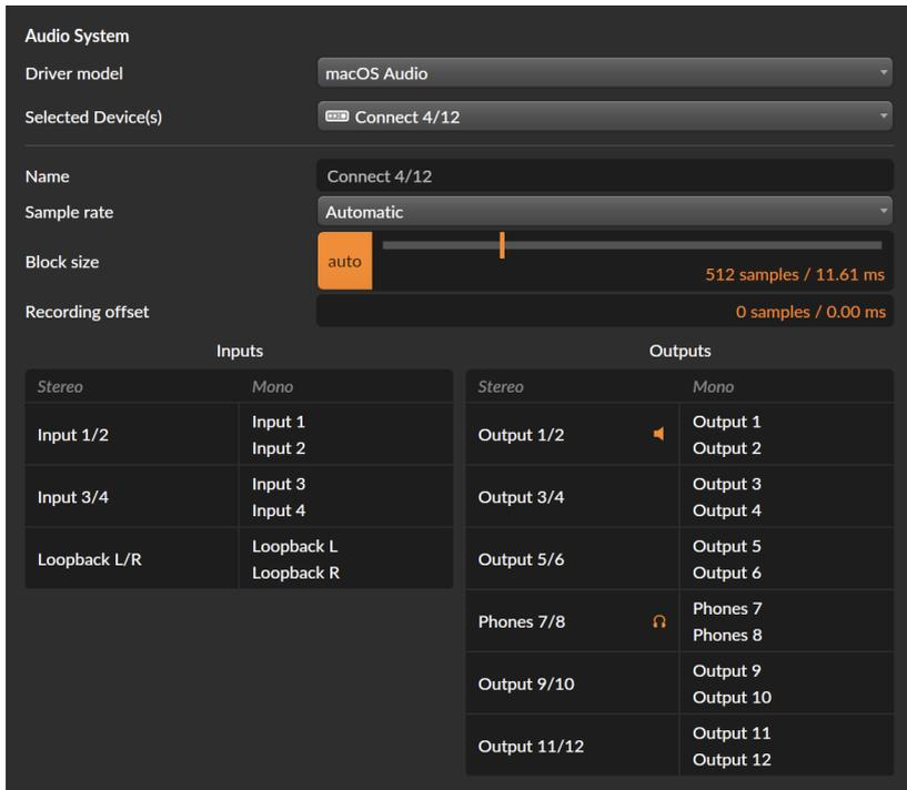
If you are using macOS or Linux, you can increase the number of inputs and outputs by using Bitwig Connect 4/12 in combination with other audio interfaces connected to your computer. Instead of choosing Connect 4/12 as your selected device, open the device menu and select *Create New Combined Device*. A list with available audio interfaces will appear below the chooser. Select the audio interfaces you want to use.
