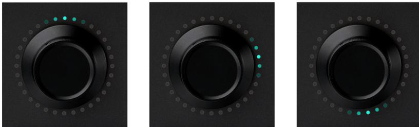
When Scroll mode is already activated, press the SCROLL button again to switch to Zoom mode. Two or more ring LEDs will light up in violet. Turn the Center Dial clockwise to zoom in horizontally, or counterclockwise to zoom out horizontally. The number of lit up LEDs will change depending on the current zoom level: the more you zoom out, the more LEDs will light up.
