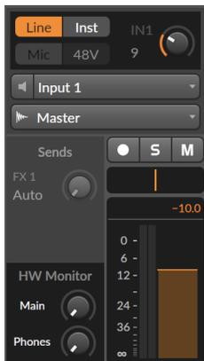
When input channel 1 or 2 is selected, you can toggle the input type, toggle phantom power (only on channel 1), and adjust the gain. When input channel 3 or 4 is selected you can toggle the DC filter and the +12
