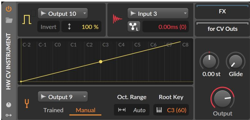
Insert a **HW CV Instrument** device on an instrument track and switch to *Manual* tuning mode. Select one of the Outputs 9 to 12 as the *Pitch*
